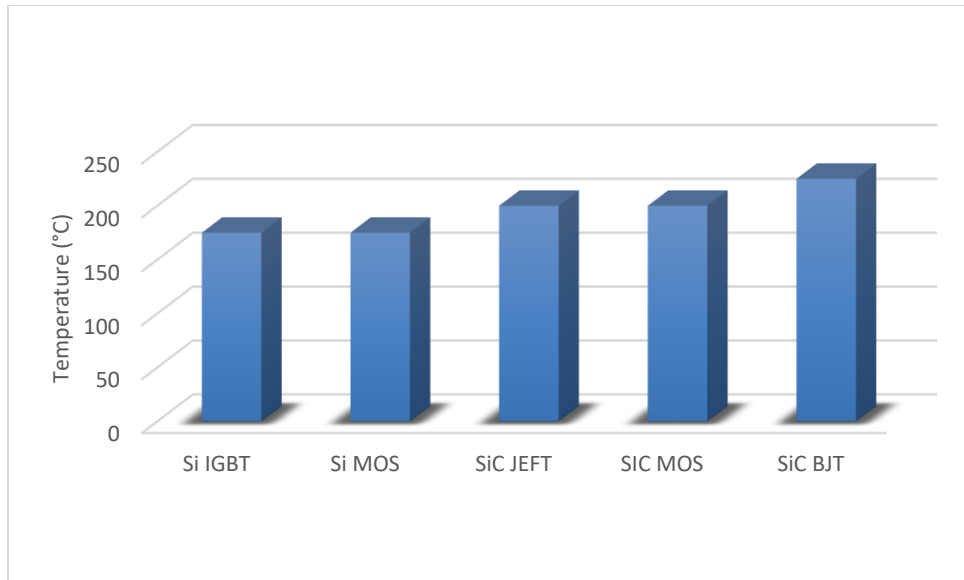
Figure 7: Maximum endurance operating temperatures of Si and SiC devices in market
